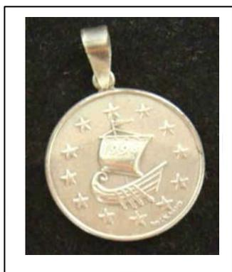
Fig. 1 Silver medaillon coated with Paraloid B72 added with 2% Al<sub>2</sub>O<sub>3</sub> nano-pigments after 1 year exposure to the atmosphere
